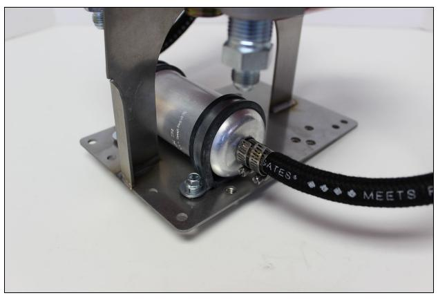
FIGURE 2 – FUEL PUMP MOUNTING & FUEL INLET HOSE CONNECTION
