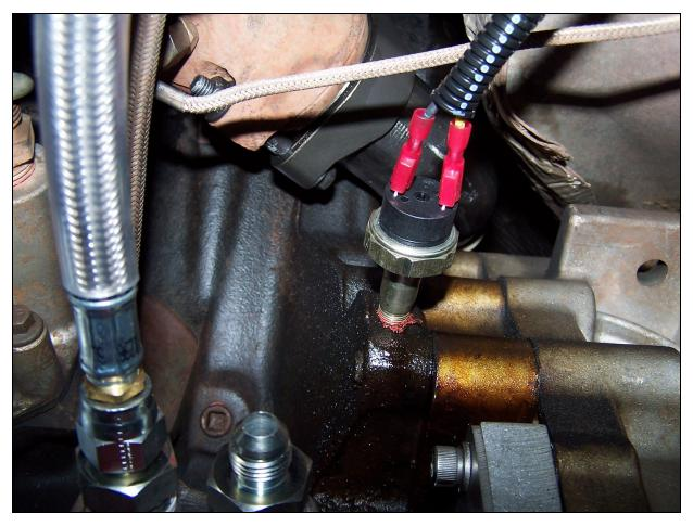
FIGURE 9 – OIL PRESSURE SWITCH INSTALLED – DRIVERS SIDE OF ENGINE BEHIND OIL FILTER
