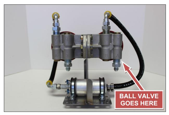
FIGURE 4 - FUEL FILTER FITTING LOCATIONS AND HOSE ROUTING - BALL VALVE NOT SHOWN
